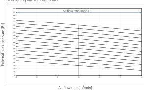
Upper limit of ESP by air flow auto adjustment
