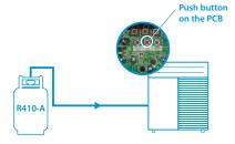
If the temperature drops below 20°C\* manual charging is necessary.
