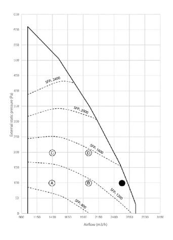
The diagram shows the available external pressure for the duct system given an airflow.
