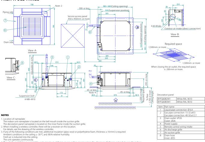
4. Though the installation is acceptable up to maximum -660-mm square ceiling opening, keep the clearance of -45-mm or less between the indoor unit and the ceiling opening, so that the panel overlap allowance can be ensured.
