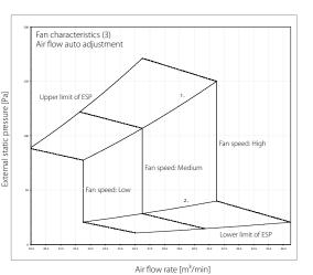
Upper limit of ESP by air flow auto adjustment
