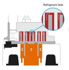
During low load, weak pressure is applied resulting in refrigerant leakage.
