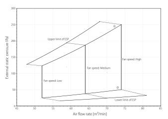
Upper limit of ESP by air flow auto adjustment
