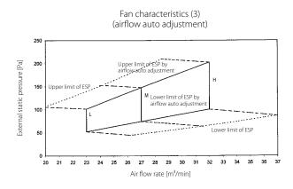
Fan characteristics (2 (Field setting with remote control))
