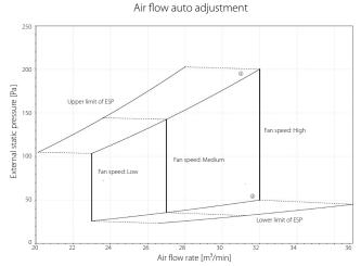
Upper limit of ESP by air flow auto adjustment Lower limit of ESP by air flow auto adjustment
