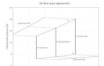
Air flow rate [m³/min]
