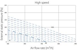
1. The fan curves are determined with  $\cdot 1/3 \cdot$  of the ESP on the outdoor side (EA & OA·), and  $\cdot 2/3 \cdot$  of the ESP on the indoor side (RA & SA).
