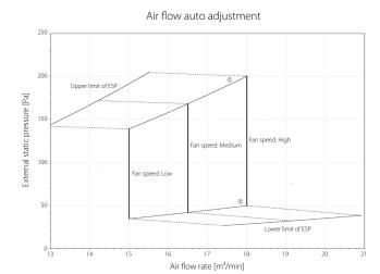
Upper limit of ESP by air flow auto adjustment Lower limit of ESP by air flow auto adjustment
