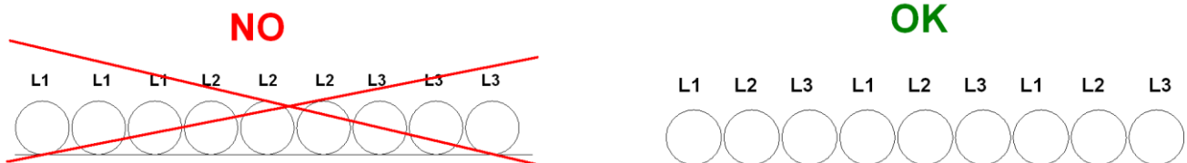
Fig. 1 - Installation of long power supply wires
