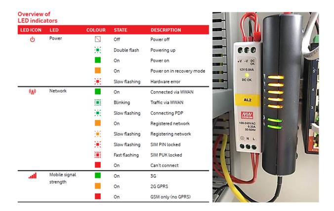
In some cases, it could be temporary solved by a **restart the modem** (by disconnecting and reconnecting its own power supply connector.
