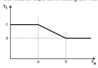
T<sub>t</sub> Target leaving water temperature
