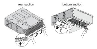
2 Clean the air filter. Use a vacuum cleaner or wash with water. If the air filter is very dirty, use a soft brush and neutral detergent.
