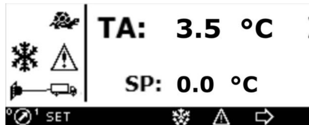
Figure 11 - "External power supply mode" operation screen
